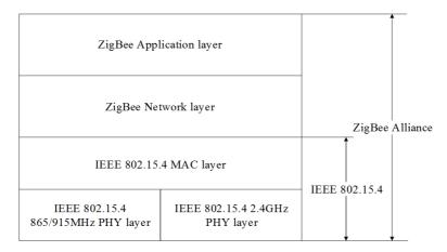
Fig. 1. ZigBee structural system diagram
